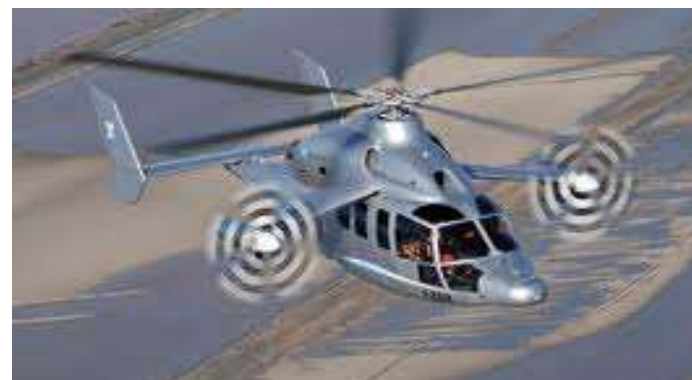
Airbus Helicopters X3 Development: 2010-2013, max 255 kt, \mu \sim 0.7
