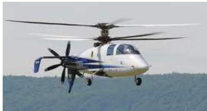
Sikorsky X-2 Development: 2008-2010, max 250 kt, \mu \sim 0.65
