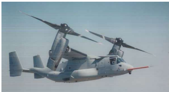
Bell-Boeing V-22 Osprey Development: 1982-1997 : In production: 1997~, max 275 kt, cruise 241 kt
