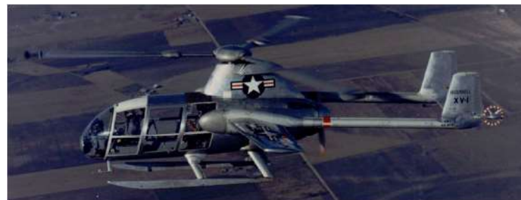
Fig. 2-4. The McDonnell Aircraft Corp., Helicopter Division's XV-1 Convertiplane. At maximum speed, the rotor operated at an advance ratio just below 1.
